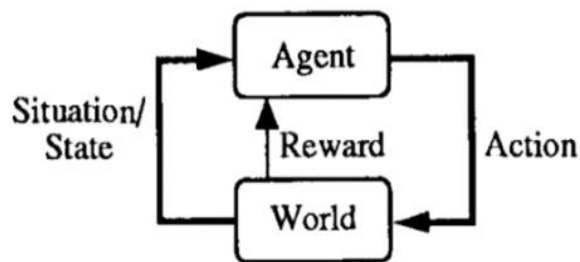
Figure 1: The Problem Formulation Used in Dyna. The agent's object is to maximize the total reward it receives over time. 1
